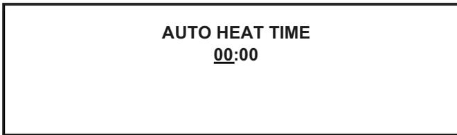
Select the arrow keys to increase or decrease the hour to the desired setting. Then move the cursor to the minutes position by pressing the SEL key. Adjust the setting for minutes, then select the SEL key to save the setting and return to the AUTO HEAT TIME screen. Select the SEL key to exit the screen and return to the Manager’s Menu.
