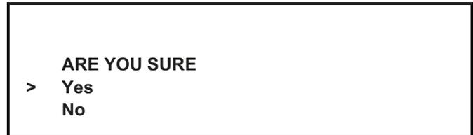
Use the Up or Down arrow key to move the cursor to "Yes." Press the SEL key to immediately start a Heat cycle.
