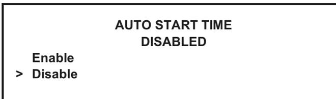
Enable the AUTO START TIME can by selecting the Up arrow key to move the arrow up to “Enable.” Press the SEL key to advance to the next screen.
