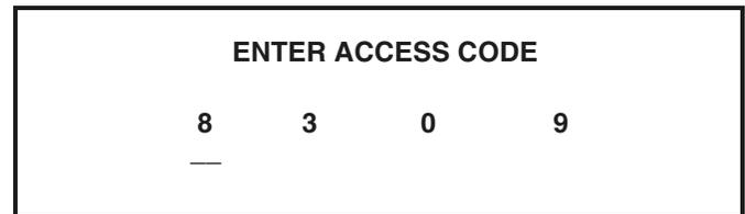
Continue to enter the proper access code numbers (8309) until all four numbers are displayed, then press the SEL key. The Manager's Menu list appears on the screen, provided the correct access code is entered.
