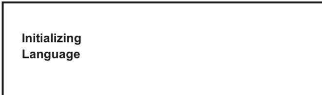
**Note:** *If there is a language initialization fault, the machine forces a language selection prior to the initializing sequence. The standard menu LEDs should light as if they were in a menu. If a language has been selected, the machine is powered down, and the machine should not ask for a language unless there is another language initialization fault. English is the factory default setting.*
