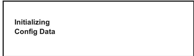
If configuration data is corrupted, all user and service settings are set to defaults. A CONFIG CRC ERR fault is displayed on the VFD. The system continues to operate in its previous mode, but with default settings.
