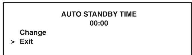
Use the arrow keys to program the auto standby time by increasing or decreasing the hour setting above the cursor. Press the SEL key to advance the cursor and program the minutes setting. Press the SEL key to return to the previous screen with the new time setting displayed. Press the SEL key to exit the screen and return to the Manager’s Menu.
