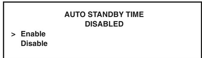
Program the auto standby time by pressing the Up arrow key to move the arrow to “Change.” Press the SEL key to advance to the next screen.
