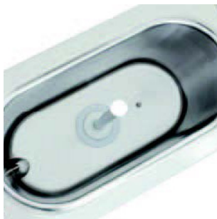
Cylinder-block vat and steel beater.
