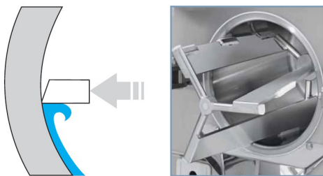
Beater with removable mobile scrapers
