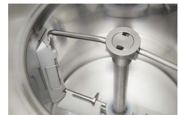
Heater agitator with removable scrapers
