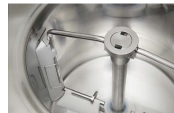
Heater agitator with removable scrapers
