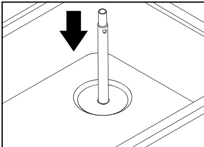
Figure 5-1 Feed Tube Position during Standby Operation
