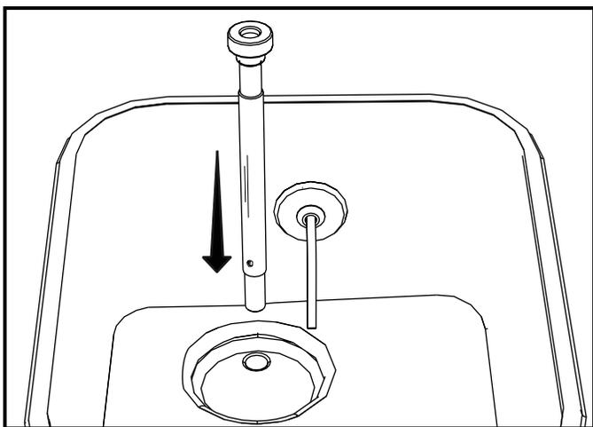
Figure 5-4 Feed Tube Position during Normal Operation
