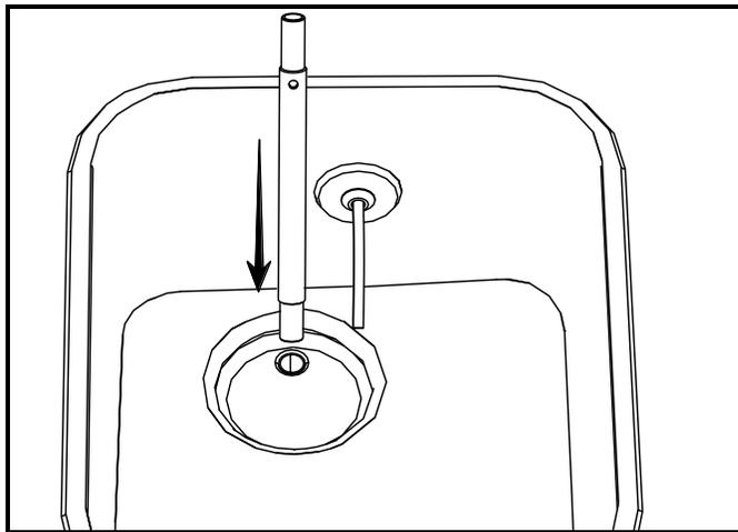
Figure 5-5 Feed Tube Position during Standby Operation
