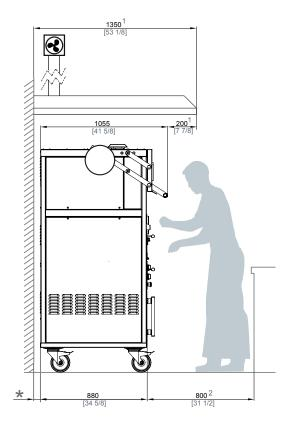
\* MINIMUM DISTANCE TO FLAMMABLE ELEMENTS: 300 mm [12 in] / RECOMMENDED DISTANCE TO ANOTHER ELEMENTS: 100 mm [4 in]
