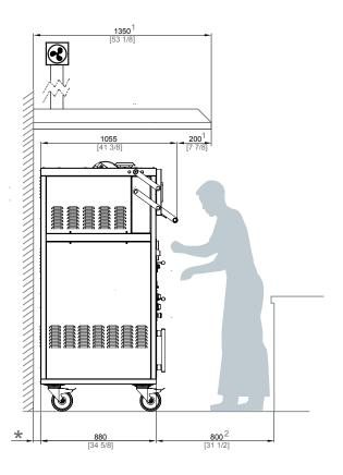
\* MINIMUM DISTANCE TO FLAMMABLE ELEMENTS: 300 mm [12 in] / RECOMMENDED DISTANCE TO ANOTHER ELEMENTS: 100 mm [4 in]
