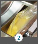
Place the vacuum bag inside the vertical chamber.
