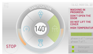
Sanitising washing (CIP + SIP)
