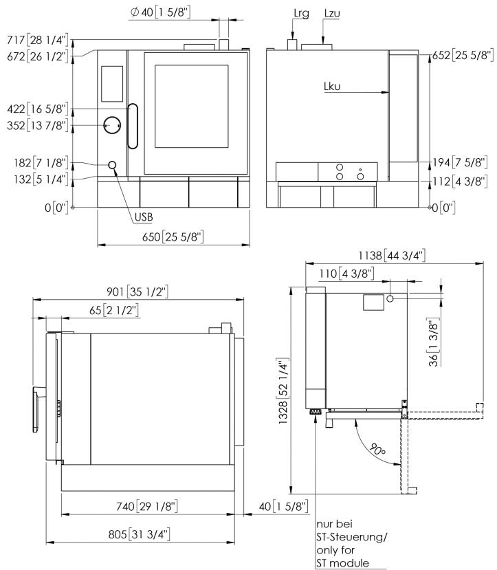
Dimensioned drawing 6-11, door stop on the right, control on the left
